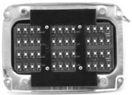
Squeeze the primer tube to break the glass bulb and wet the brush end with primer. Rub the primer on the lenses and the housings at the places where the tape will touch. Treat both left and right housings and lenses at the same time before the primer tube dries out.
